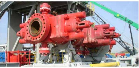
The Wrangler system enables safer and more efficient assembly, transportation, and installation of BOP stacks.
