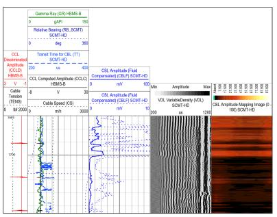
In a Thailand field known to have annular pressure problems, wells cemented after conditioning with CemPRIME Scrub spacer experienced no such problems (from SPE-180624).
