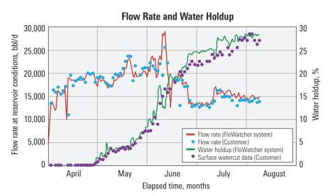
Downhole flow rate and water holdup data acquired over several months by the FloWatcher system correlated closely with the customer's independent measurements of flow rate and surface water cut taken at the surface.
