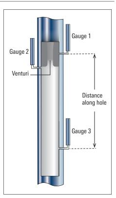
FloWatcher flow rate, fluid density, and PT monitoring system.
