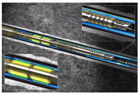
HEWM hydraulic and electric downhole wet-mate connector.
