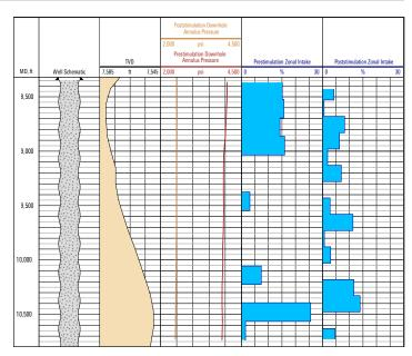
Comparison of pre- and poststimulation injection profiling along the openhole horizontal section. The acid stimulation targeted the middle section and resulted in a more uniform water injection distribution along the open hole. Surface injection pressure was reduced from 1,000 to 0 psi.
