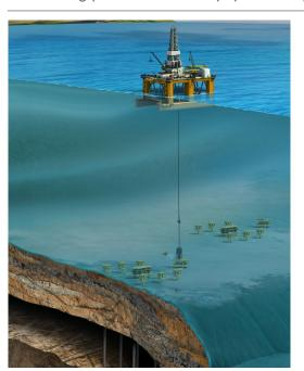
Coil Tubing Services, a Schlumberger company, proposed CT riserless operations in P&A wells after the zonal and casing packer isolation had been successfully set and tested. Engineering and operational evaluations were performed to address CT string integrity, bottomhole assembly, surface CT stack rig-up, remote operating vehicle use to string the CT into the wellbore, CT depth correlation, cement slurry design, and proper fluid placement.
