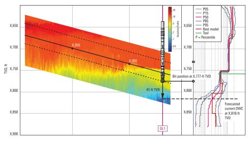
The IriSphere service detected a low apparent resistivity trend ahead of the bit by 41 ft from last bit position.
