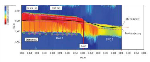
An operator improved well path location in relation to reservoir fluids using the HDS service. When combined with reservoir-scale mapping from the GeoSphere service, the top and oil/water-contact (OWC) boundaries were further optimized.
