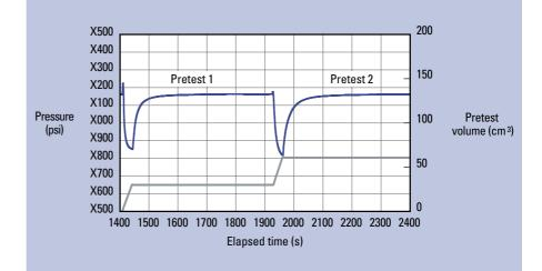
To verify integrity of the plug after the plugging operation, the pressure is reduced below the formation pressure and monitored to check the plug seal.
