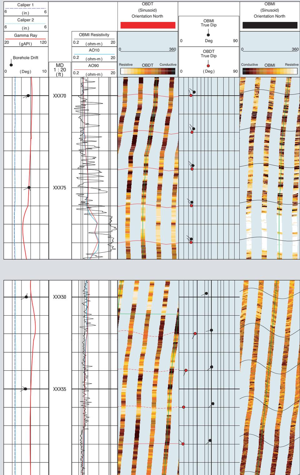
OBMI images and quantitative  $R_{xo}$  measurement from a deepwater well in the Gulf of Mexico show an excellent match to the ultraviolet-light core photograph and conventional logs. Thresholds are applied to the OBMI  $R_{xo}$  data to calculate the net pay thickness in the far-right track.
