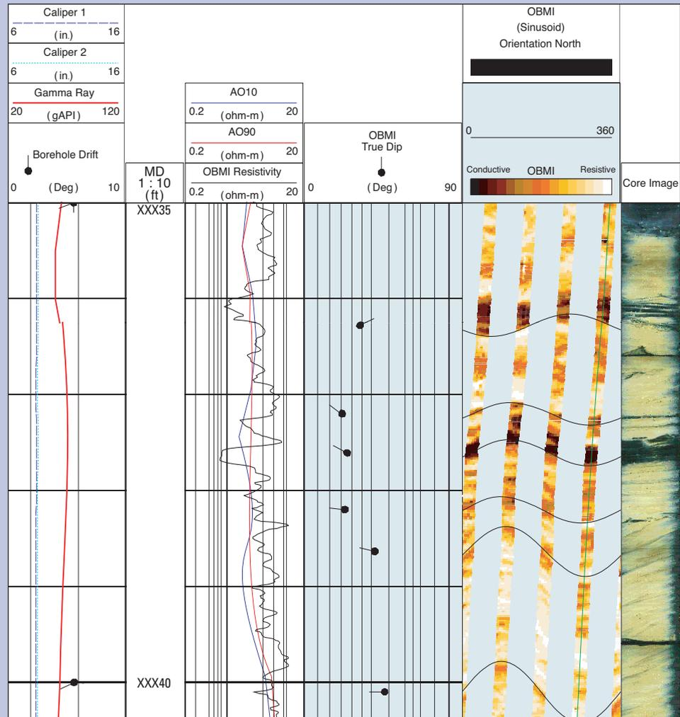
The OBMI image provides a structural overview of the bottom of a pilot hole for a horizontal well in the Alberta Foothills, confirming the target between XX52 and XX60 m. The accuracy of the OBMI  $R_{xo}$  measurement is verified by excellent correlation with the shallow AIT\* Array Induction Imager Tool log.
