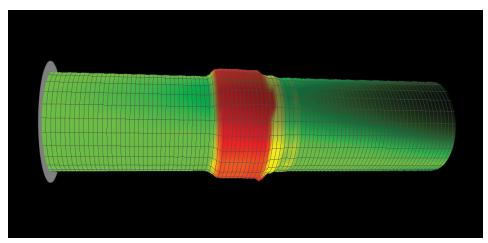
The 1-ft gap in the tubing indicated in red on the image from the PipeView\* multifinger caliper tool posed conveyance risks during both descent and pulling out that had prevented deployment on slickline and on coiled tubing in the deviated well.
