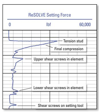
Direct measurement of the axial force applied during the plug setting operation by ReSOLVE intervention service confirmed installation.
