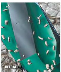
Conventional fluids allow gumbo buildup and bit balling to occur, slowing down the entire drilling process.
