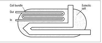
Salt bath heater filled with eutectic salt surrounding the coils. The fire tube is immersed in the steam bath heater's water bath, with the coil above the water level.
