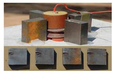
Test shows the controlled explosive energy generated by a PowerCutter tool.
