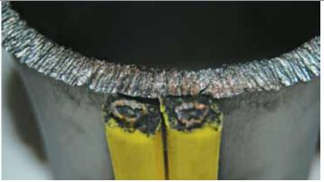
Because the PowerCutter tool produces a clean cut (left), the pipe remaining downhole is much easier to retrieve than pipe having the characteristic "open-flower" cut resulting from conventional explosive cutters. Both tubing and control lines are cleanly cut (right).
