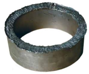
The high-quality cut of this 5½-in 26-lbm/ft 25% chrome tailpipe was obtained with the 4.15-in PowerCutter tool, which can pass through a 4.25-in subsea safety valve.
