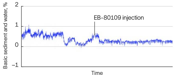
Injection of the new demulsifier stabilized and reduced the basic sediment and water level in oil to 0.3%–0.5%, suitable for export.
