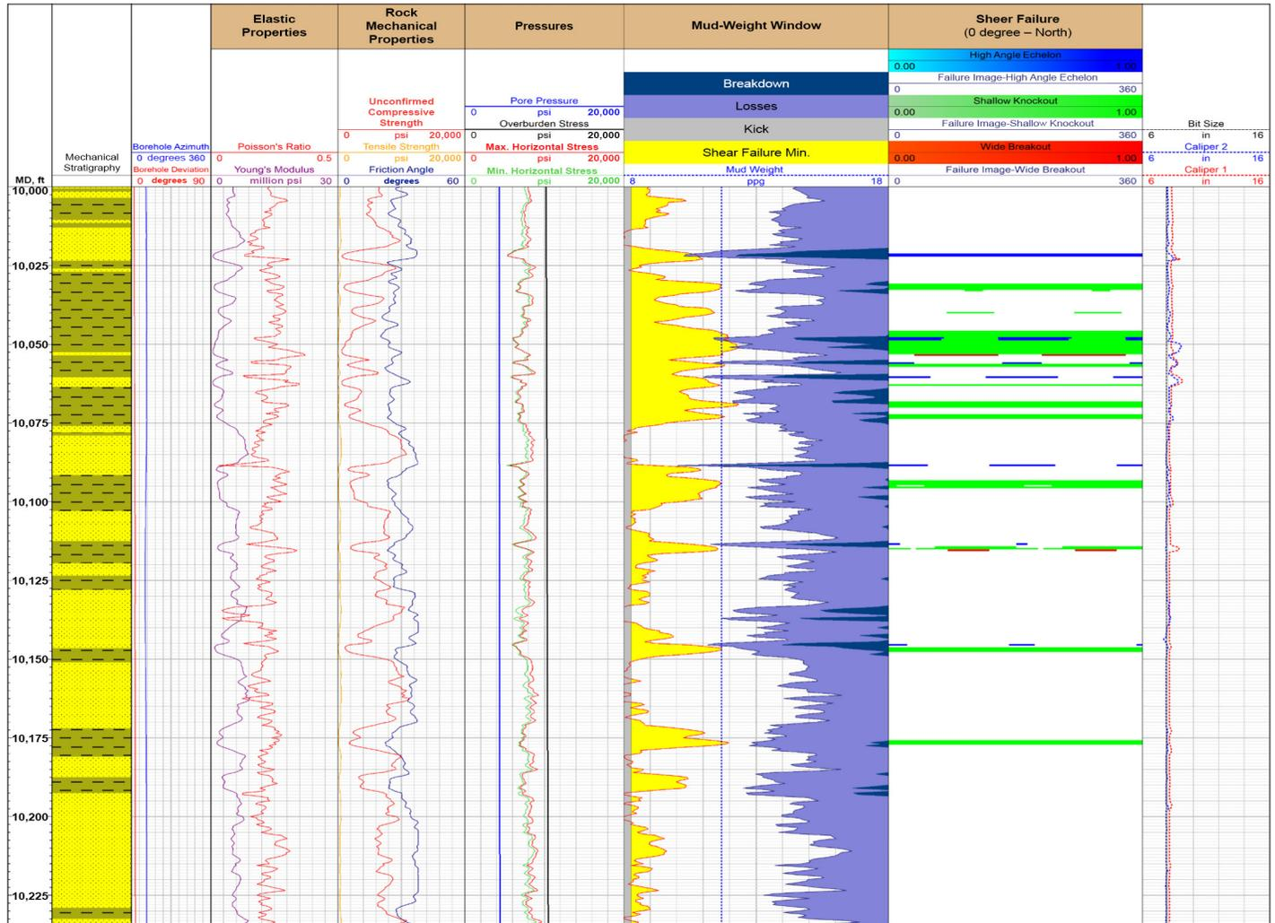
Mechanical earth model showing wellbore stability analysis for single trajectory.
