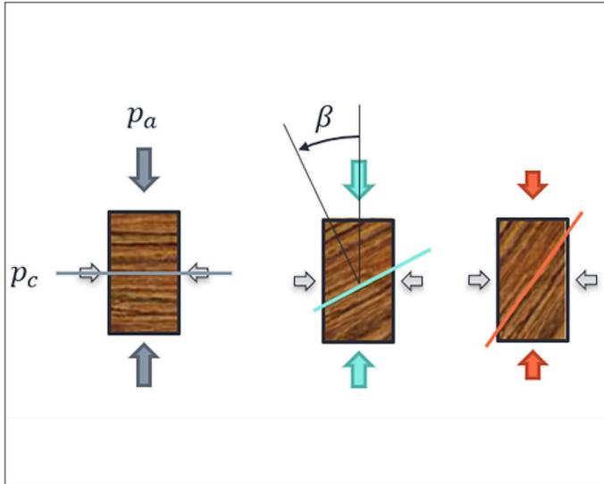
Plane of weakness failure analysis with rock strength measurements at various angles to the bedding planes.
