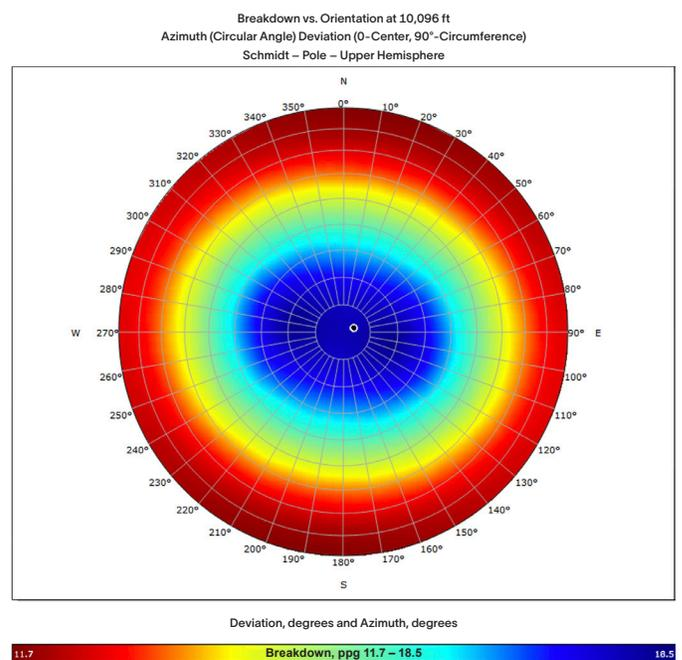
Breakout mud weight vs. orientation.
