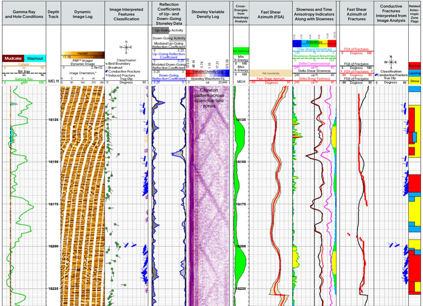
Integrated fracture characterization composite plot displaying extensive open-fracture zones.
