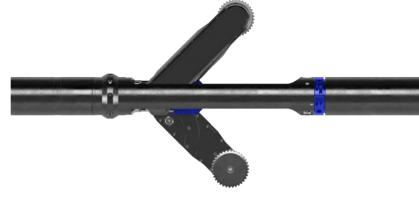
The TuffTRAC iX tractor seamlessly runs with any SLB cased hole services, including powered ReSOLVE<sup>™</sup> instrumented wireline intervention services and WIReD devices in both the 31/8- and 21/8-in sizes. WIReD devices can be run above or below a TuffTRAC iX tractor to increase fishing capacity. The critical systems of head tension and gamma ray or active casing collar locator (CCL) logging are already built in to the tractor.
