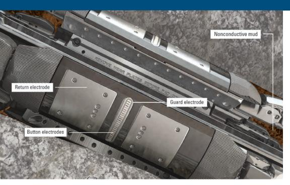
Quanta Geo service achieves high-definition imaging by applying 192 microelectrodes at high vertical and horizontal resolution.
