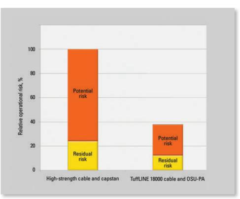
TuffLINE 18000 cable deployed using an OSU-PA offshore unit reduces both potential and overall operational risk by more than 60% compared with conventional operations using high-strength cable and a capstan.
