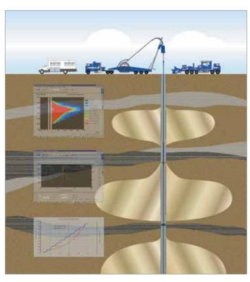
The CoilFRAC stimulation service offers flexibility in fracture design and placement by taking into account varying formation characteristics such as stress contrast, permeability, porosity, and fracture gradient.
