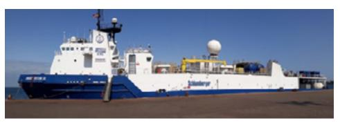
DeepSTIM II stimulation vessel delivers high-volume, high-rate, and high-pressure fracturing, acid, and sand control operations for operators in West Africa.
