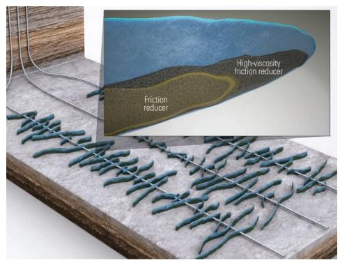
Visualization of sand settling under dynamic flow conditions indicates that a viscous slickwater fluid transports proppant more efficiently compared with a conventional friction reducer as evident.
