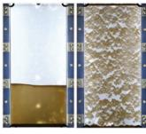
▲ Comprising a blend of proprietary fibers and rheology-controlled fluids, Schlumberger composite fluids promote effective proppant transport and placement through the formation of highly conductive channels.
