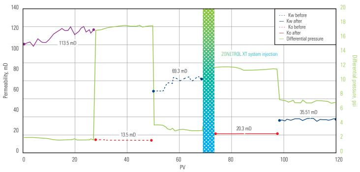
In this instance, the ZONETROL XT system increased the permeability to oil (Ko) by 48% while effectively reducing the permeability to water (Kw) by nearly 49%.
