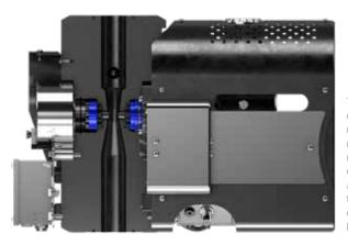
The Vx Spectra flowmeter contains a venturi section with multivariable transmitter for measuring total flow rate; a nuclear source and detector that obtain oil, gas, and water holdups; and a compact flow computer that performs all calculations and converts flow measurements from line to standard conditions.
