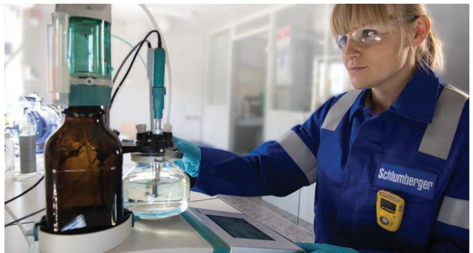
*Automatic titration following ASTM International UOP 212 procedures allows for faster, more reliable analysis of sulfur compounds.*
