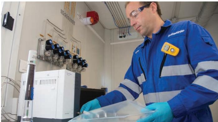
The fully portable MicroGC with an integrated thermal conductivity detector enables quick and accurate measurement of  $C_1$ - $C_7$  hydrocarbons,  $CO_2$ ,  $N_2$ , and  $H_2S$  down to 50 ppm.
