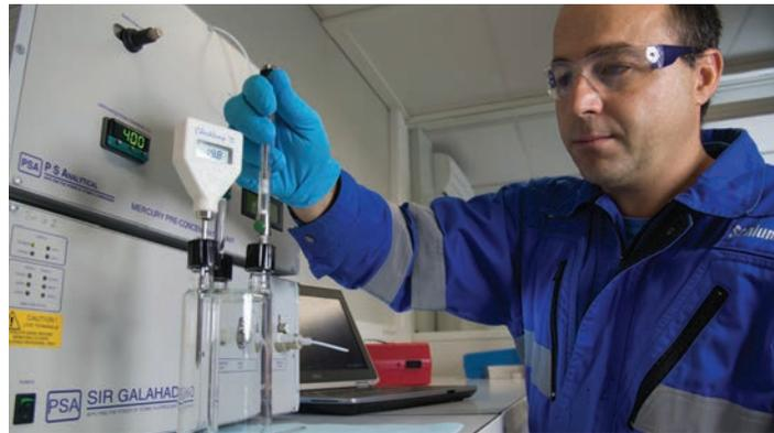
Field-proven, industry-standard Sir Galahad equipment is used to detect mercury content in gas down to 1-ng/m<sup>3</sup> concentration levels.
