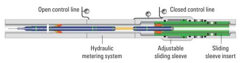
Sliding sleeve and ReSOLVE iX service schematic.
