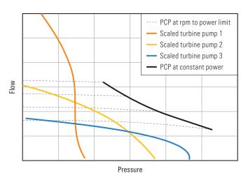
Comparison of PCP for the debris removal application to the industry standard.
