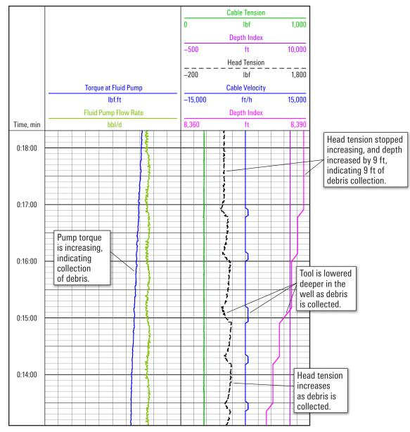
ReSOLVE iX service real-time measurements of cable behavior, indicating effective debris removal.
